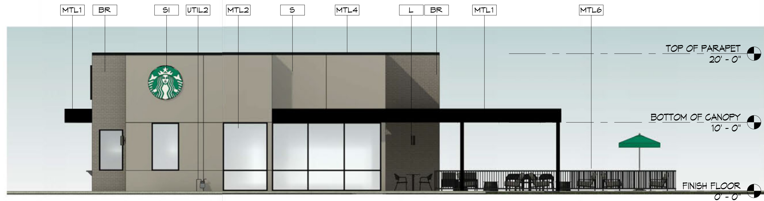
1 EAST EXTERIOR ELEVATION 1/8" = 1'-0"
